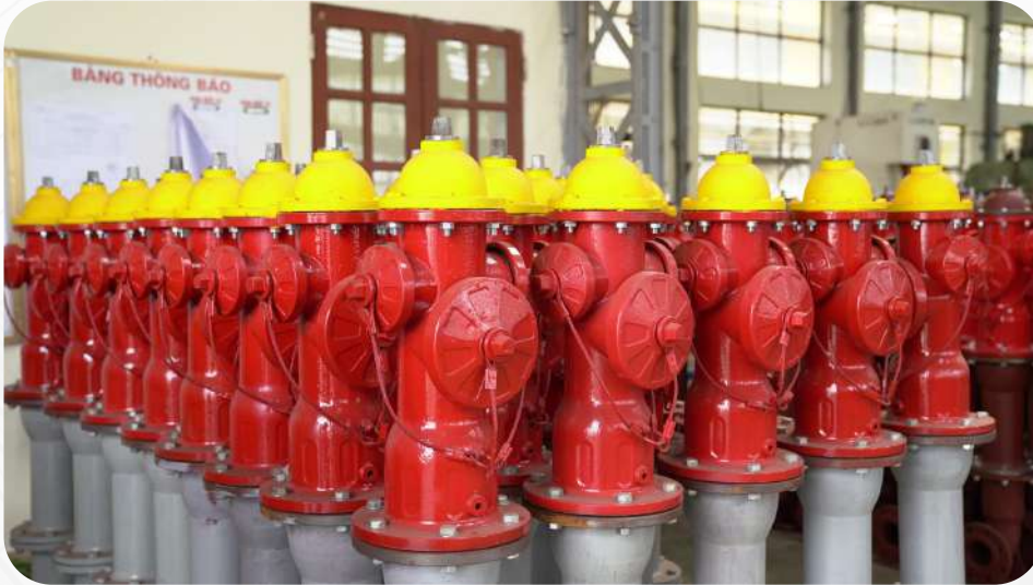
3 NOZZLES FIRE HYDRANT
